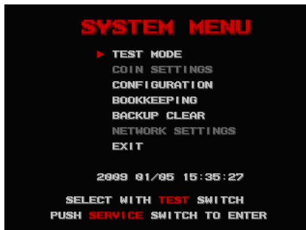
Use the TEST Button to move the cursor and the SERVICE Button to select. It is impossible to select gray items (COIN SETTINGS and NETWORK SETTINGS).
