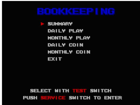
Move the cursor to “EXIT” after checking operation status and press Service Button to return to System menu.
