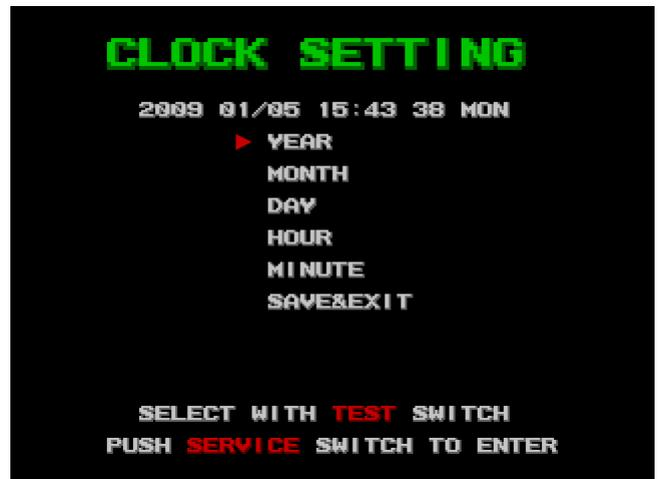
Move the cursor to “SAVE&EXIT” after setting change is complete. Press SERVICE Button to return to SYSTEM menu after setting is saved.
