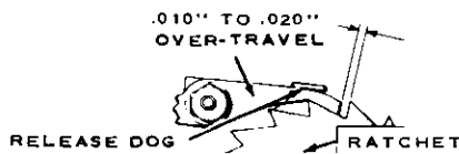
Figure 3. Release Dog Over-Travel Detail.
