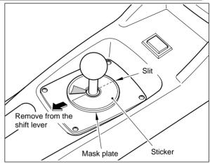
•The mask plate is used again after replacement of the shift unit. Keep it in a safe place.
