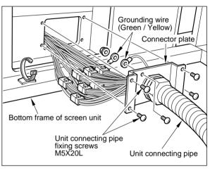
To separate the screen unit and the projector unit
