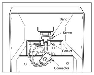
Take the reverse steps to install the button into position. If the socket has been replaced, reconnect the cables as shown below.
