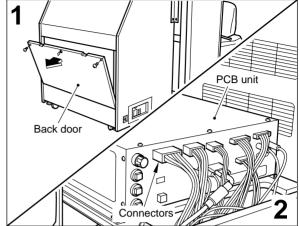
Remove the thumbscrews and take out the PCB unit together with its wooden board.
