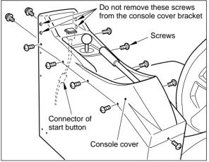
Remove the screws. Take out the hand brake unit and disconnect the connector.
