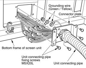
Fix the unit connecting pipe with the nylon band that is located at the bottom frame of the screen unit.
