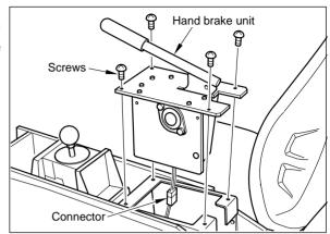
Disconnect the wiring and the ground wire from the potentiometer. Remove the screws and take out potentiometer bracket.
