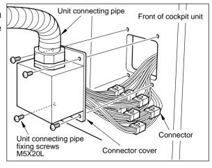
To disconnect the unit connecting pipe
