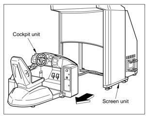
Remove the connector cover from the cockpit unit. Disconnect all the connectors.
