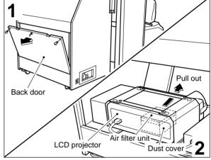
Pinch the projection of the filter presser with your fingers. Flip up the holder and take out the air filter.
