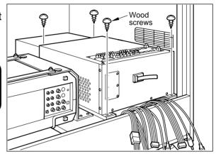
Remove the screws and detach the air filter cover.
