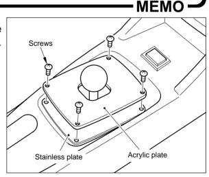
Remove the screws. Pulling the hand brake toward yourself, detach the console cover and its bracket (see page 54). Also disconnect the connector of the START button.
