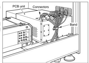
Remove the screws and take out the PCB unit.
