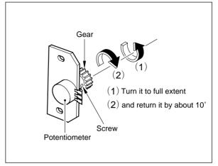
Mount the potentiometer bracket, paying attention so that the gear B should be engaged with the gear A provided at the hand brake unit.
