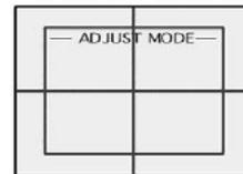
Make adjustment so as to have red superimposed on green. When red is superimposed on green, the color becomes yellow.
