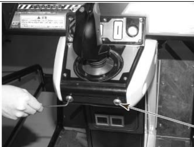
HEXAGON SOCKET SCREW (2) M4x12, spring washer, special washer used
