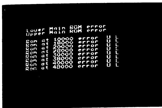
Figure 2-1 ROM Test Fails
