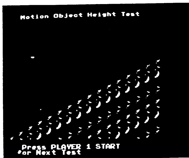
Figure 2-11 Motion Object Height Test
