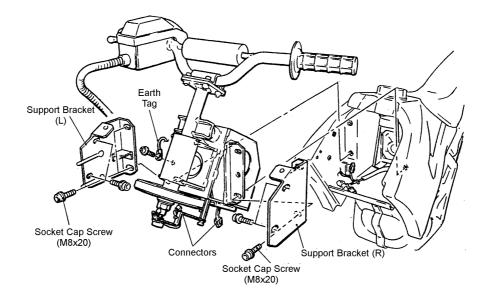
Note: When placing the handle bar assembly on to a surface, ensure that no weight is placed on the Potentiometer.
