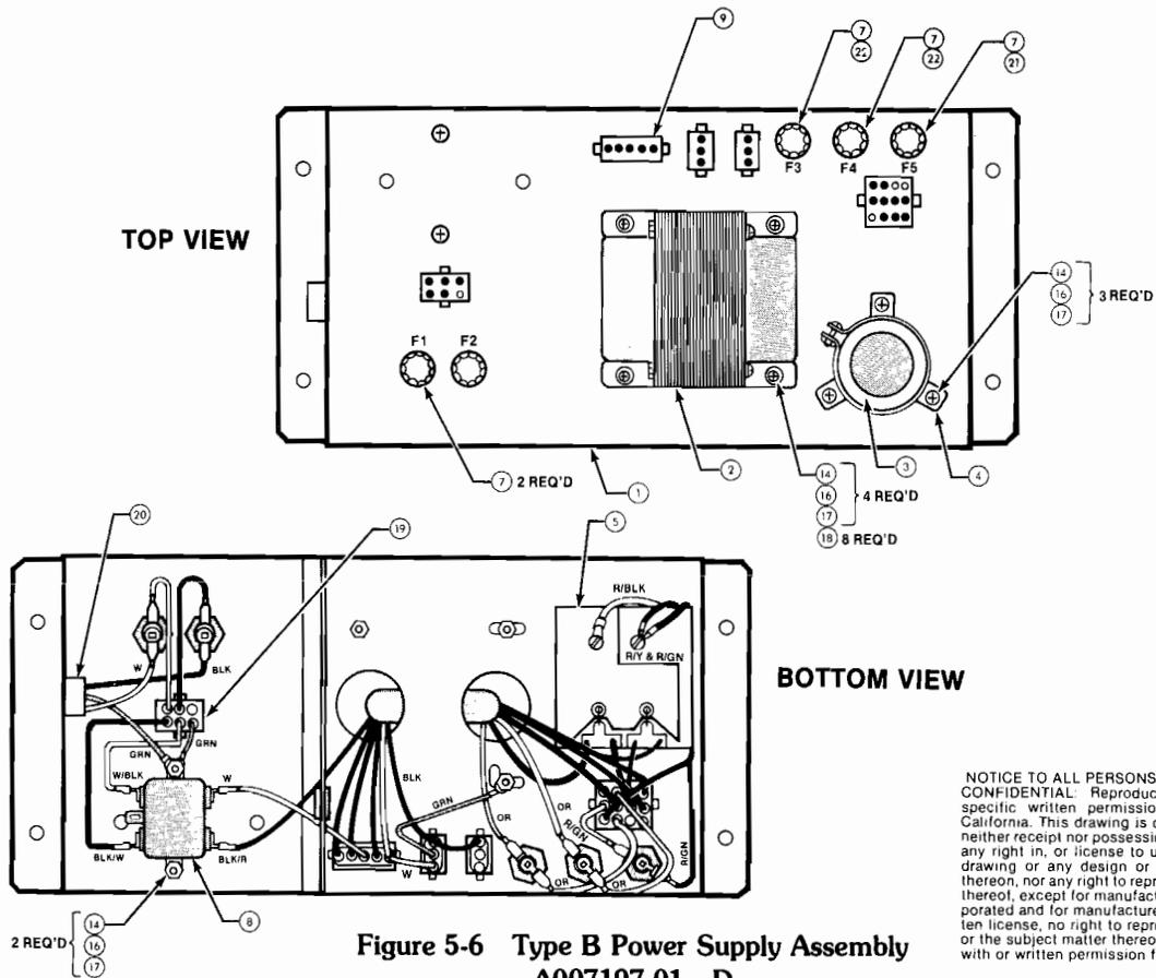
Figure 5-6 Type B Power Supply Assembly Parts List
