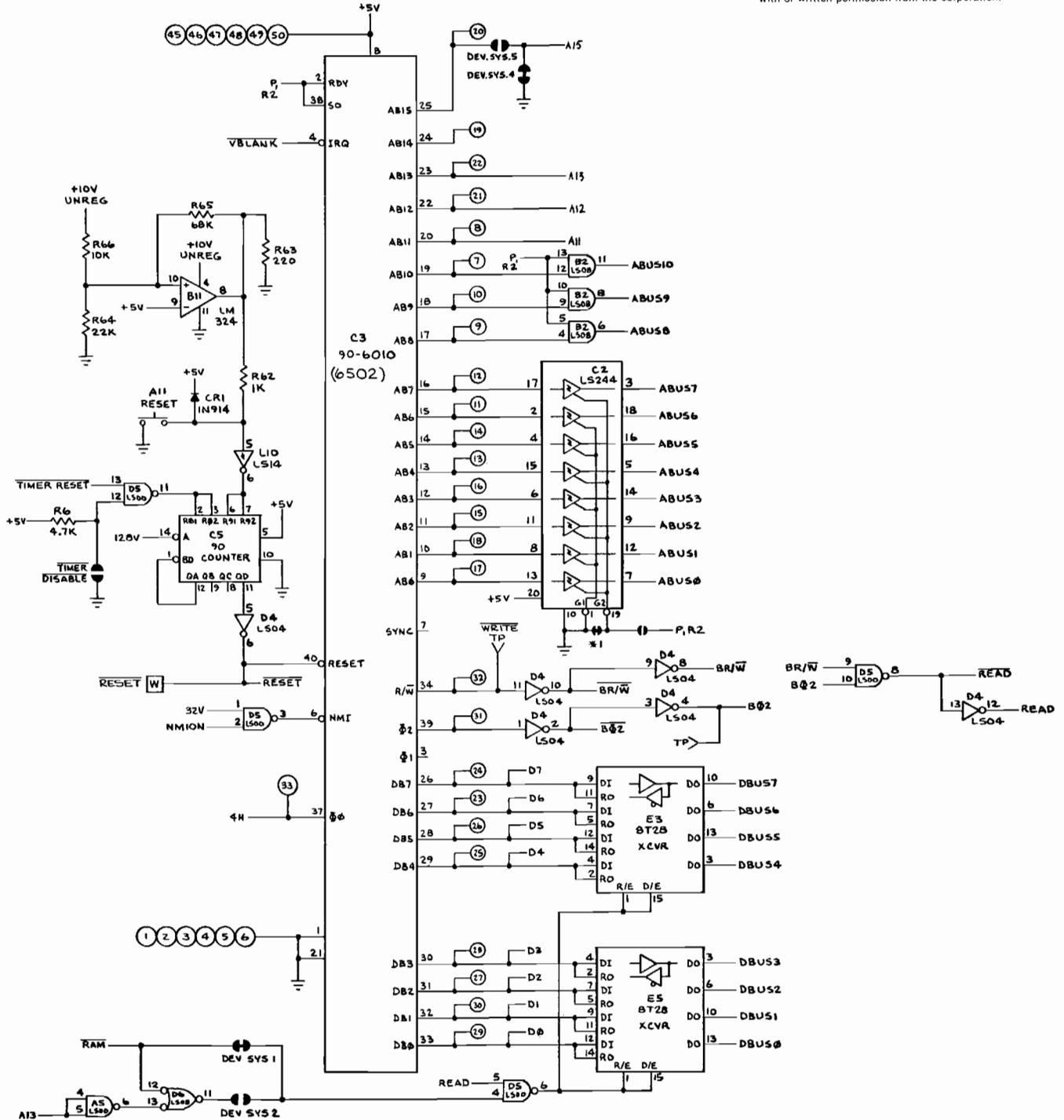
Figure 4-5 MPU Circuit Schematic Diagram
