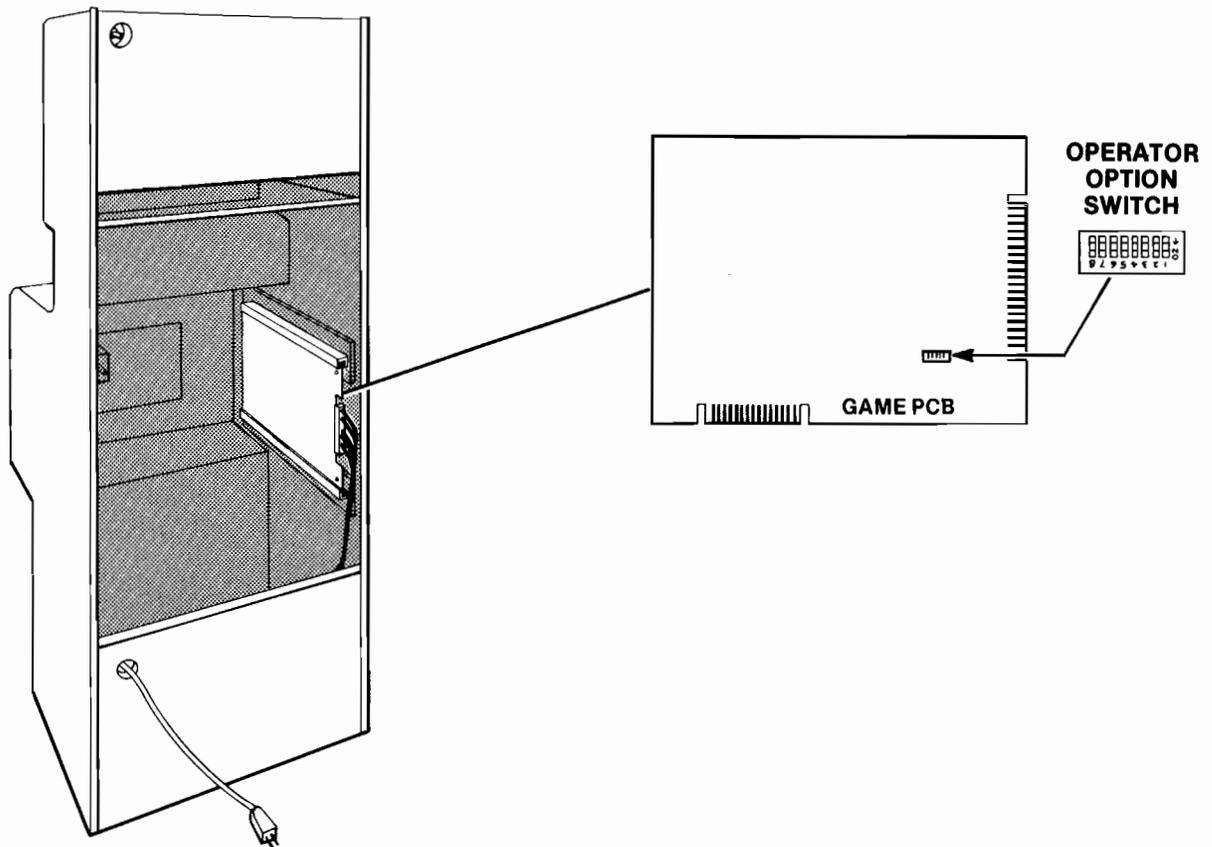
Figure 1-5 Operator Option Switches
