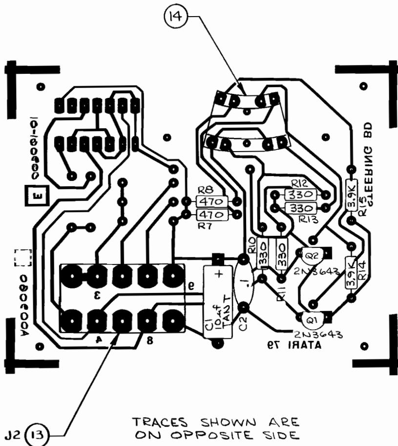
Figure 5-5 Steering Board Assembly
