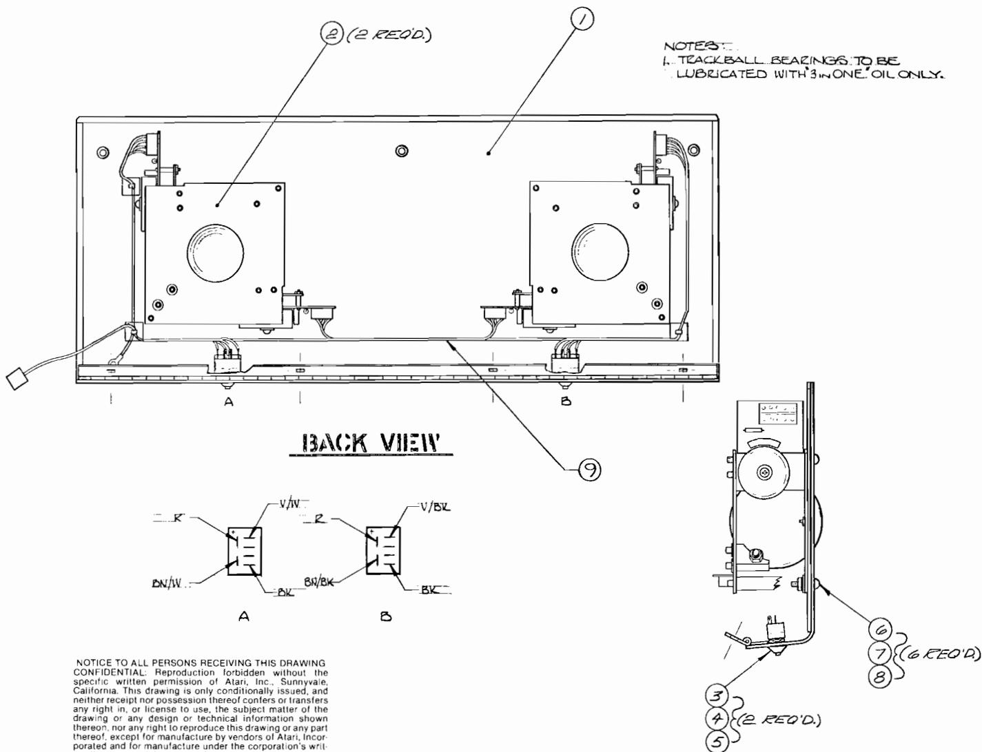
Figure 5-3 Control Panel Assembly
