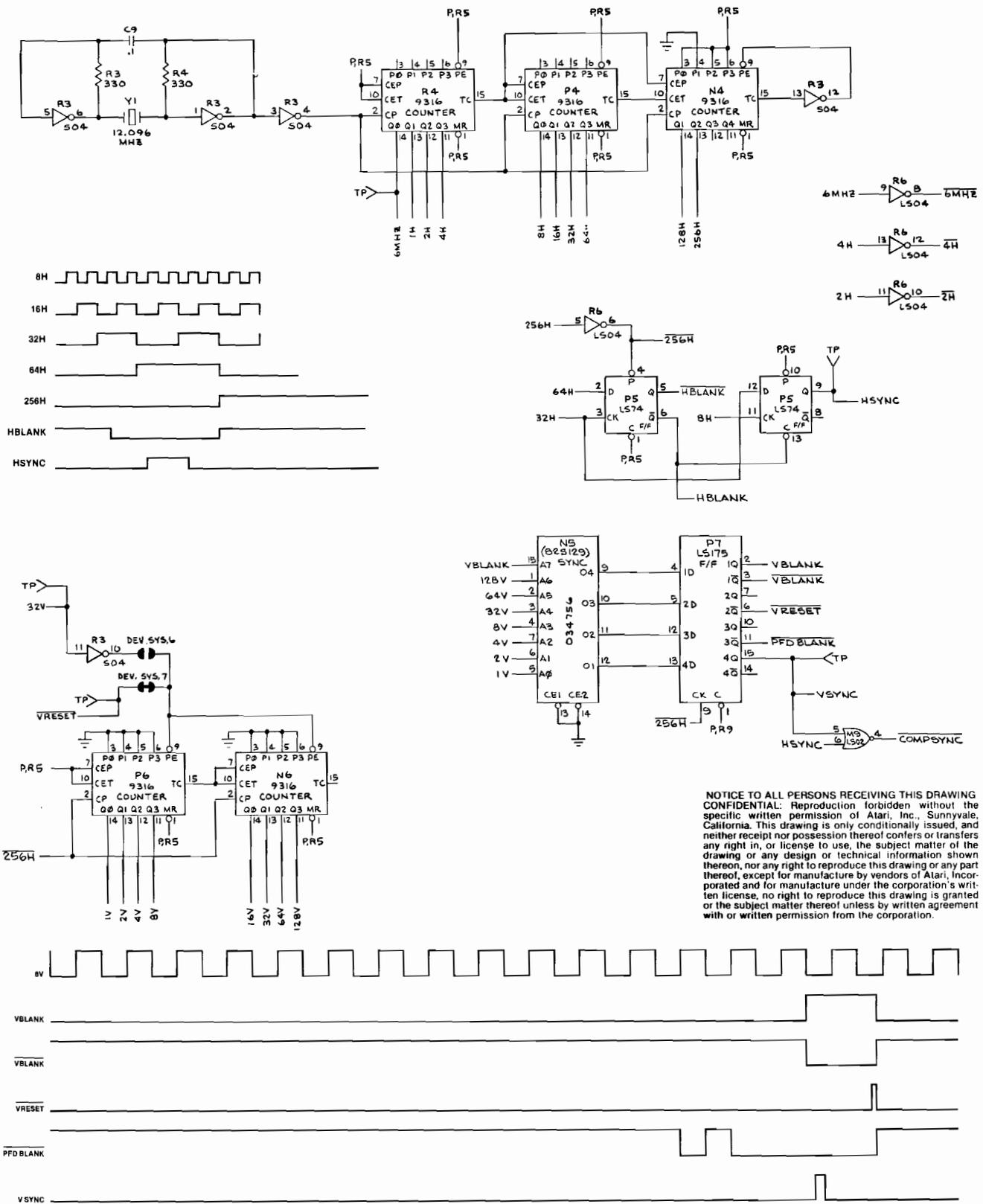
Figure 4-9 Sync Generator Schematic Diagram
