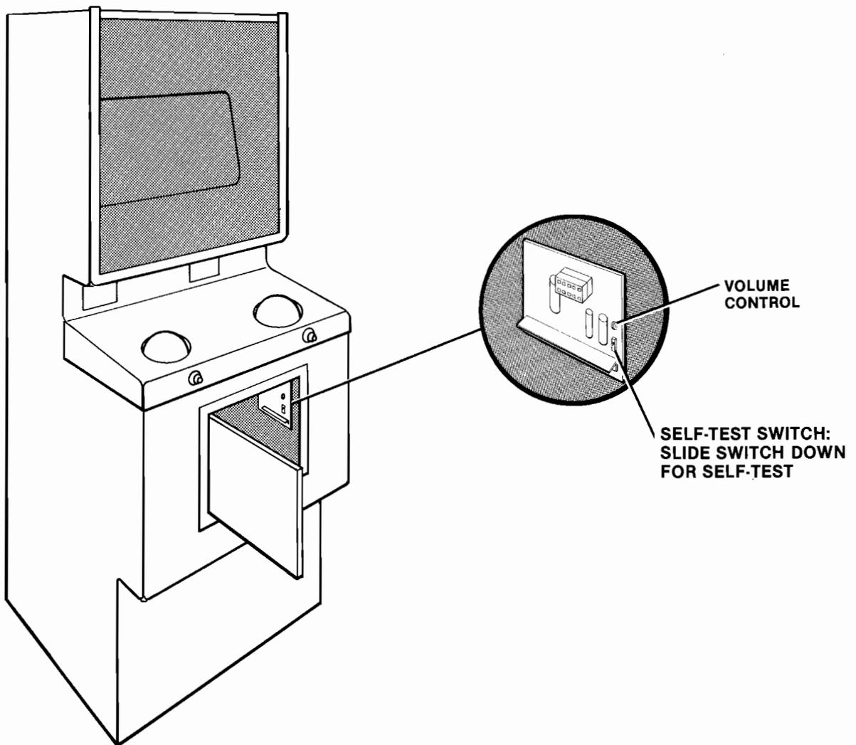
Figure 1-4 Volume Control and Self-Test Switch
