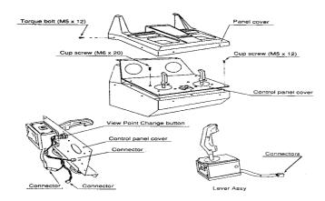
2. Remove seven hex head bolts (M5 x 20), then the control panel cover together with the Lever Assy.
