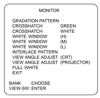
3. Lean the bike to select a test and press 'View Change' to enter the test and to return to "Monitor Menu" from a test.
