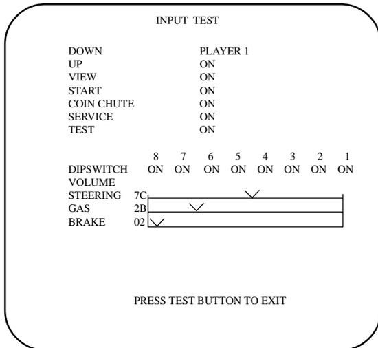
Selecting the INPUT TEST on the Test Mode menu screen causes the screen (on Which each switch and V.R. are tested) to be displayed. Press each switch. For the coin switch test, insert a coin from the coin inlet with the coin chute door being open. If the display beside each switch indicates "ON", the switch and wiring connections are satisfactory. Check the display of V.R. value for steering wheel and accelerator & brake. If the V.R. values are not satisfactory, make adjustments as necessary.
