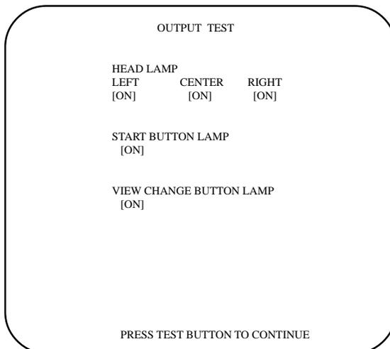
In the OUTPUT TEST mode, carry out lamp test to ensure that each lamp lights up satisfactory.
