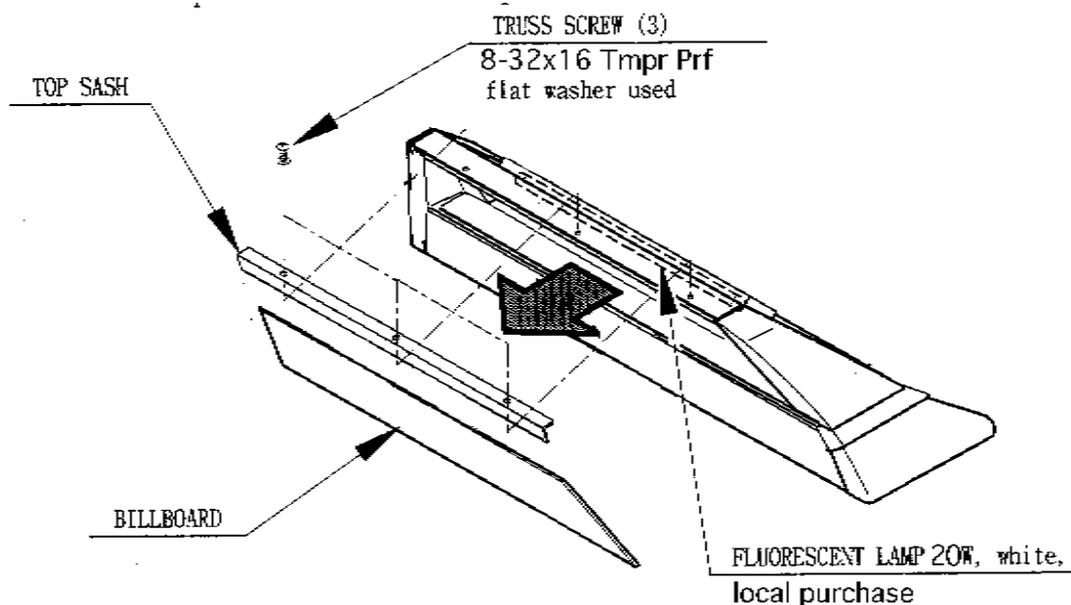
**NOTE:** To remove the the glow lamps within the lower marquee, the entire billboard assy must be removed from the cabinet.
