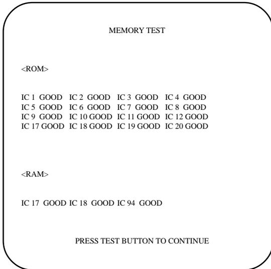
Selecting the MEMORY TEST on the test mode menu screen causes the on-board memory to be tested automatically. The game board is satisfactory if the display beside each IC No. shows GOOD.
