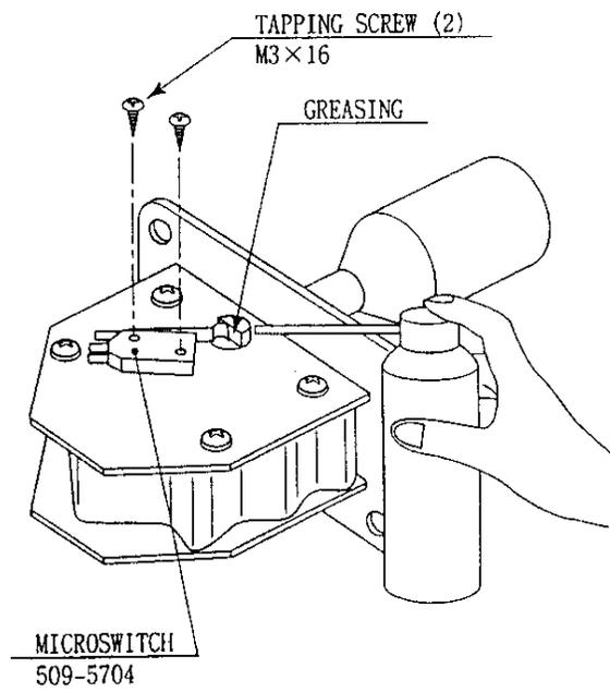
After replacing the Switch, check to see if the switch is inputted as per Shift Lever operation in the Test Mode.
