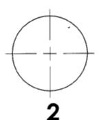
THE CENTER OF BUTTON #2 SHOULD BE LOCATED 2.75" ABOVE, AND 9" TO THE LEFT OF THE CENTER OF THE TRACKBALL.
