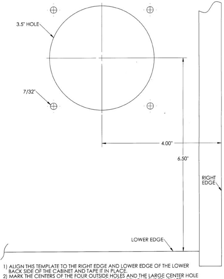
USING AN AWL, NAIL, OR OTHER SHARP OBJECT. REMOVE THE TEMPLATE.
