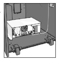
**NOTE:** The Nighthawk Chassis comes equipped with an external air filter to help keep dust, smoke and debris from collecting on the electronic components. Check and clean this filter regularly to avoid costly repairs.
