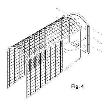
NOTE: DO NOT OVER TIGHTEN THE BOLTS IN THE PIPES, OR THE INSERTS COULD BE DAMAGED. BE CAREFUL NOT TO CROSS THREAD THE BOLTS IN THE PIPES.
