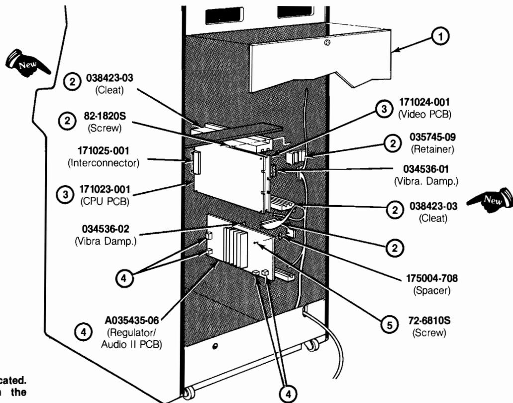
Figure 3-8 Printed-Circuit Board Removal
