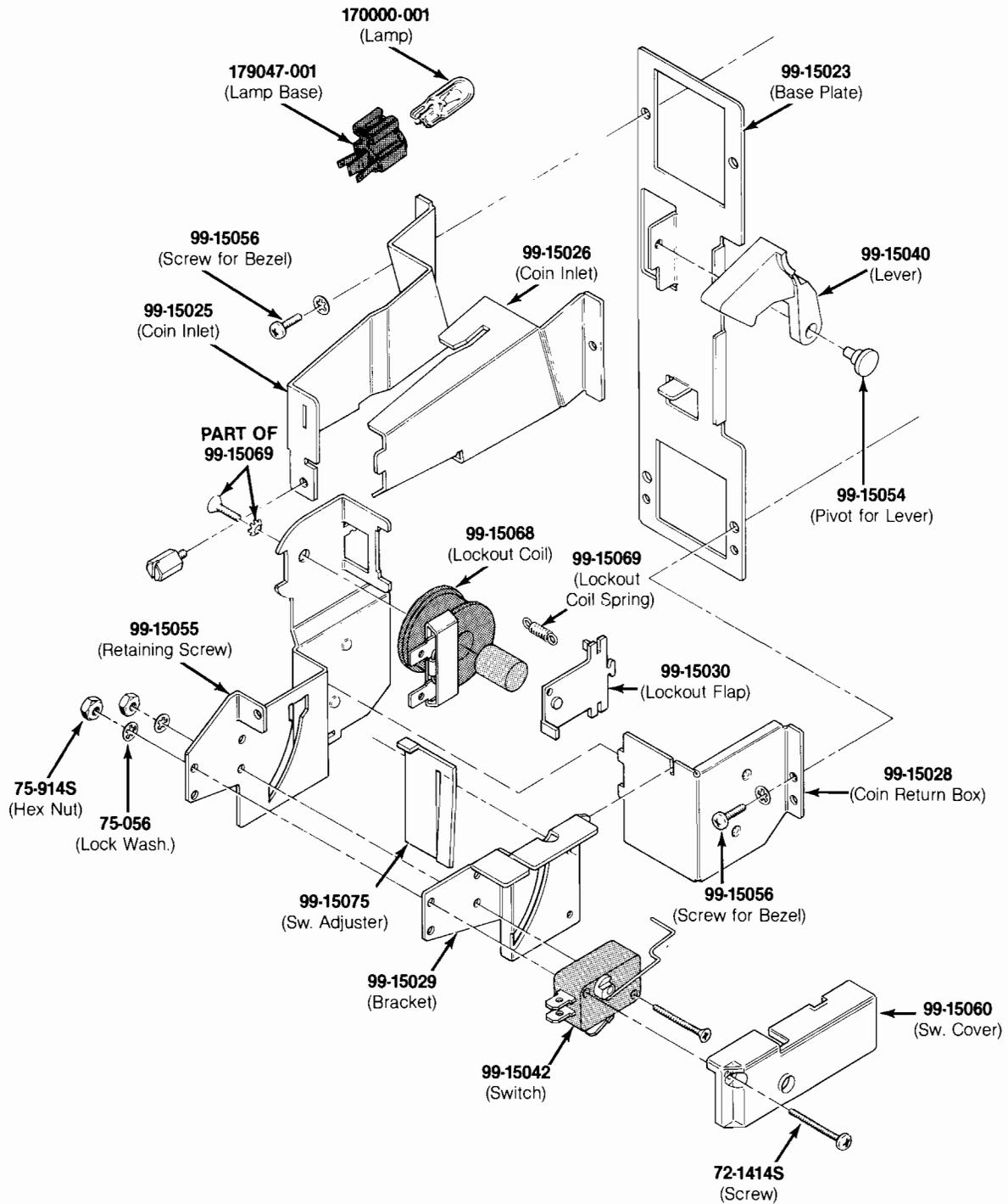
**Figure 3-7 Vertically Mounted Coin Door
