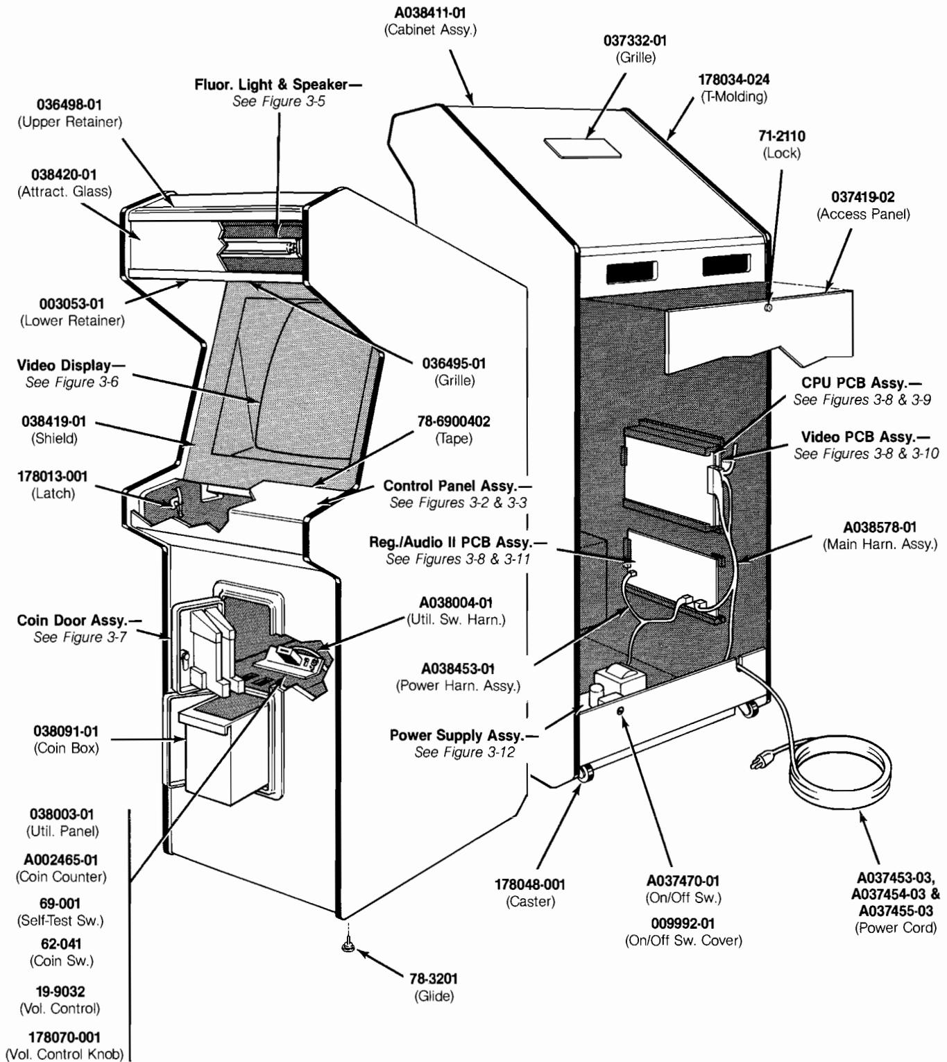
Figure 3-1 Cabinet-Mounted Assemblies
