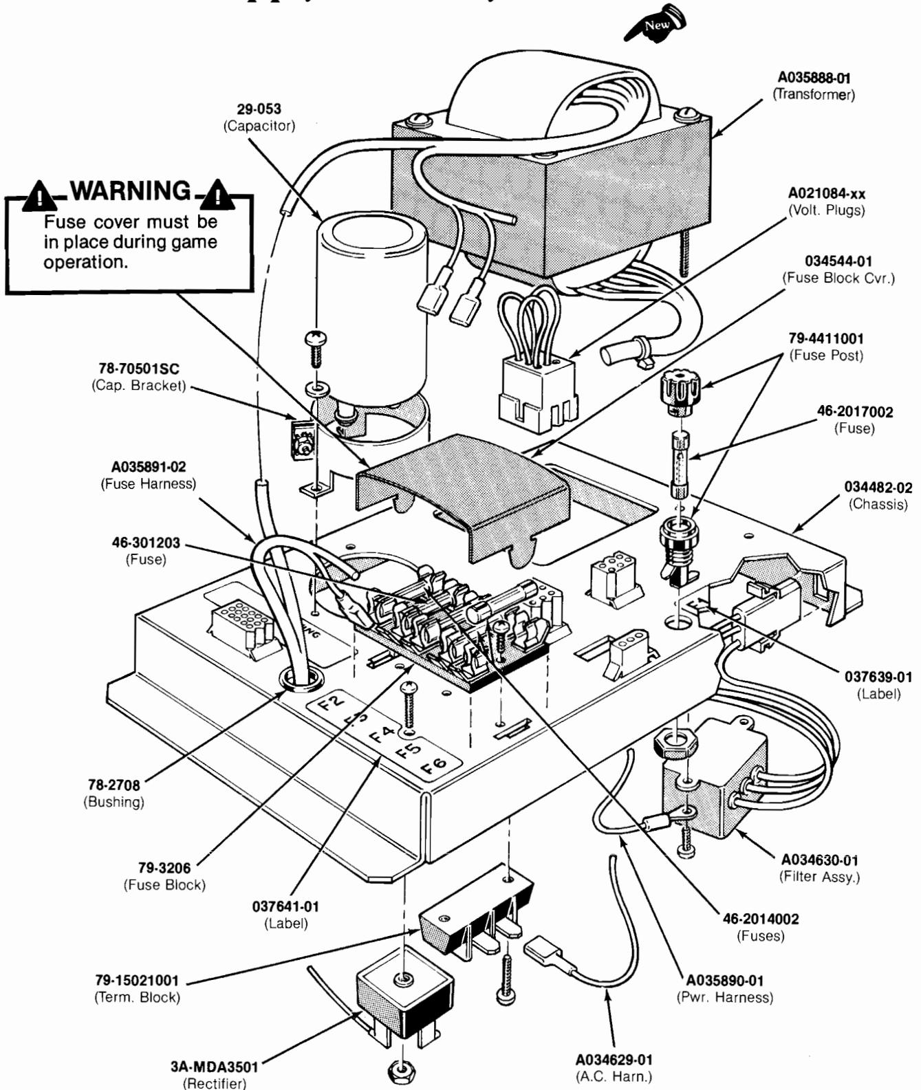
Figure 3-12 Power Supply Assembly
