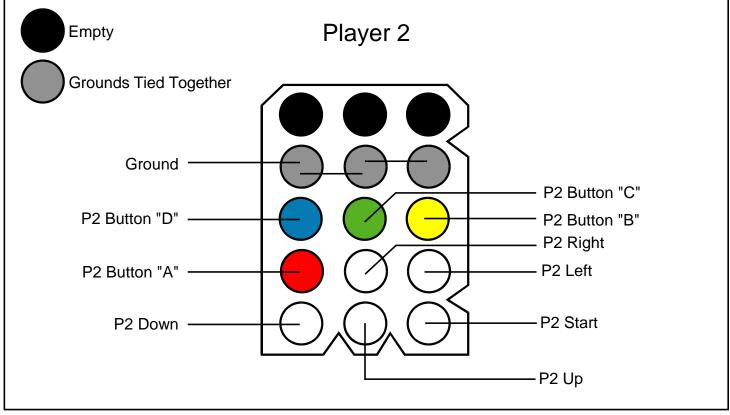
FEMALE Control Panel Connector - Jamma Edge Connector Side
