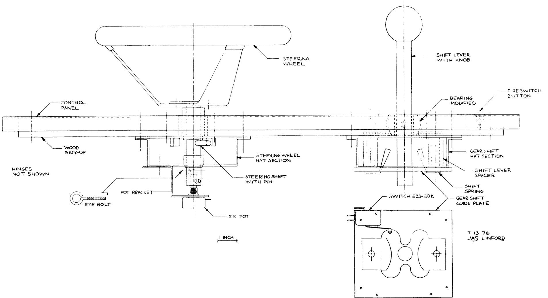
**CONTROL PANEL SCHEMATIC DIAGRAM**
