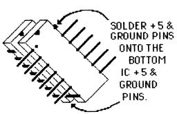
"PIGGYBACK" ONTO A 14 PIN 7400 SERIES IC ON THE BOARD AND RUN JUMPER WIRE TO AN UNUSED EDGE CONNECTOR PIN
