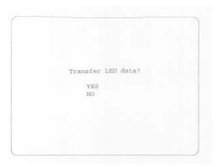
After selecting "YES" or "NO" by moving the P1:8-direction lever up and down, settle it with PI-BUTTON 1. It is automatically settled after 10 seconds approximately even if the P1-BUTTON 1 is not pressed. In any case, the item displayed in red is supposed to be selected.
