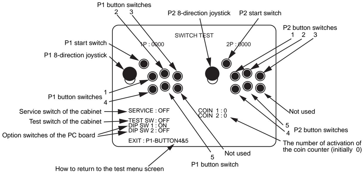
2. The Joystick on the display will move as the Player Joystick is operated. The Button Switches on the display will be highlighted as the corresponding Player Button Switch is operated. The display for the other switches will change from OFF to ON as each switch is operated.
