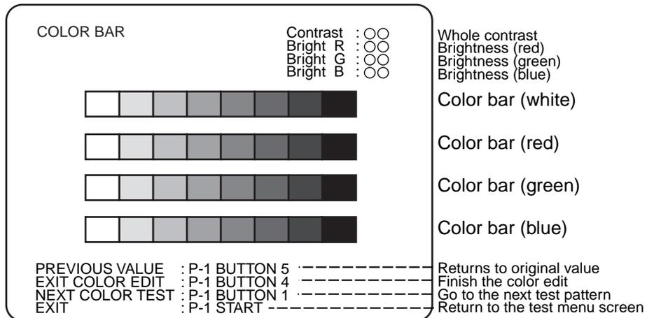
Each colour bar of 'white', 'red', 'green' and 'blue' is displayed with gradual shading. Press Player 1 Switch 2 to change the density from 32 > 16 > 8 > 4 > 2 > 32 . . . . .
