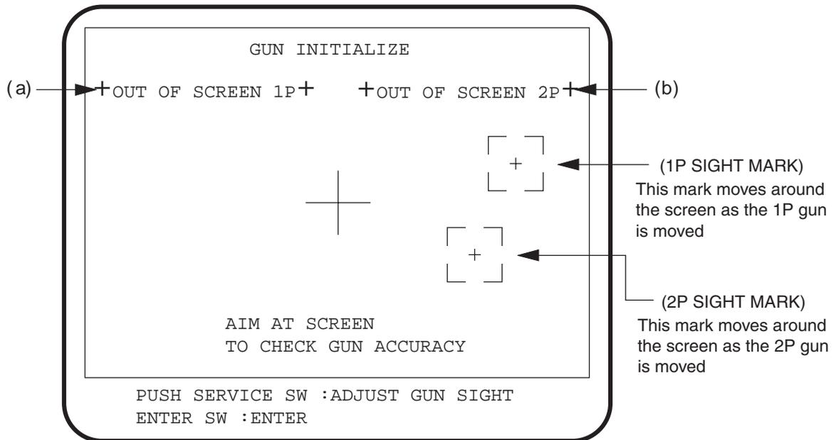
The 1P and 2P gun sights can be checked using the screen above.
