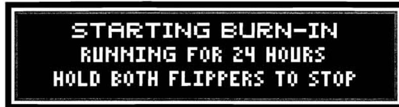
The Burn-In Test energizes all of the machine hardware in a sequenced pattern. All the solenoids are fired, motors run, and lamps flashed. The dot matrix display and sound system are also activated as well. This test is primarily intended for factory use to assure that all electronic and mechanical features are operating when the game leaves the factory.
