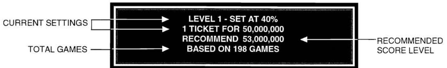
To accept the recommended new score level, press the START button. To cycle through the remaining score levels, press either FLIPPER button. To cancel, back-up, or restore the original setting, press both FLIPPER buttons simultaneously.
