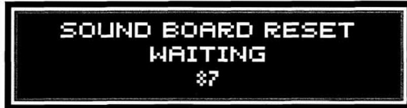
The Sound Board Test resets the sound board and causes it to report its powerup status. Press the start button to restart the test.
