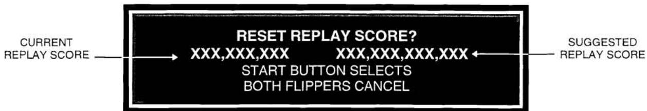
The operator can elect to accept the suggested replay score, by pushing the start button, or ignore the change in score by pushing both flipper buttons simultaneously. This action will return the system to the Main Menu. Additional information regarding Replay credits and scores can be found in the *B1 : Standard Adjustments* section of this manual.
