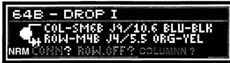
The Lamp Test will start all game lamps flashing. The flippers can then be used to get detailed information about any individual lamp. This information includes the lamp name and number, row and column information from the lamp matrix, its' wire colors, and an icon indicating whether the lamp is active.
