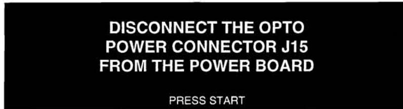
Open the backbox and remove connector J15 from the Power Board. Then, when verifying each opto, check that the opto icon does **NOT** have a vertical line (representing a “triggered” receiver condition). In this case, make sure that all balls are secure in a ball holding device (since infrared light can be reflected off the game ball) and re-test. If the opto continues to fail this test, repair/replace as required.
