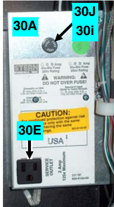
Enlarged Inside Cabinet View of Items 30: Power Box (30A), Service Outlet (30E), Fuse (30i) and Fuse Holder (30J).
