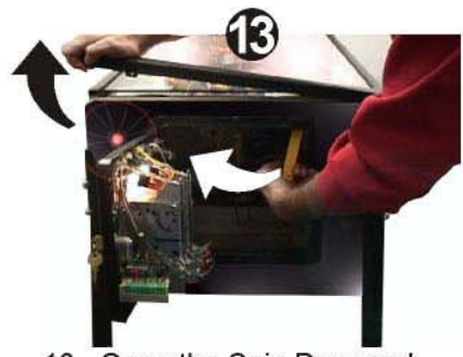
13. Open the Coin Door and pull the YELLOW HANDLE to the LEFT and at the same time pull up on the FRONT TOP MOLDING and remove. The GLASS can now be pulled out towards you and removed. TAKE CARE while moving; set glass on a safe surface.
