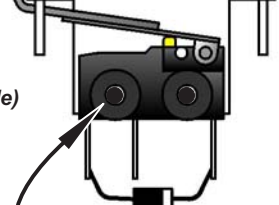
Light Force is indicated with the switch mounting studs painted black. ● Standard Force remains the natural color of the plastic bracket.
