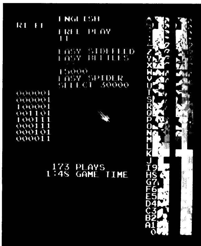
Figure 2-2 Self-Test Screen 1—Test Fails
