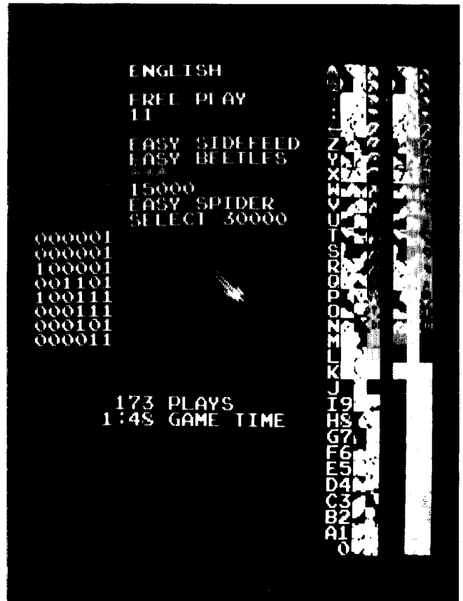
Figure 2-1 Self-Test Screen 1—Test Passes
