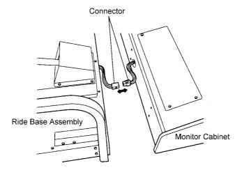
5. Disconnect the connectors and move the ride assembly completely away from the monitor cabinet.
