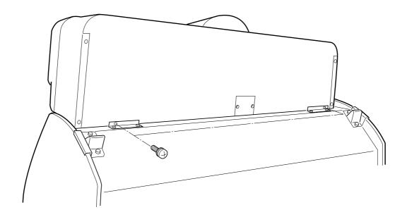
4. Slide the header assembly forward so that it disengages with the retaining bracket.
