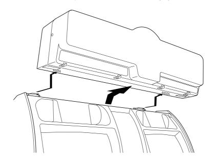
5. Remove the Header Assembly
