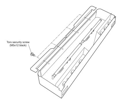
4. Fit the **new** Header Acrylic with 10off torx security screw (M5x16 chrome), supplied.
