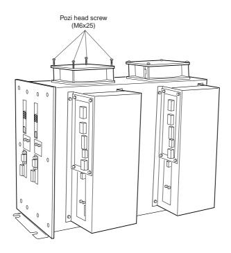
5. Fit the fans to the new Game PCB in <u>exactly the same way up</u> using 4off pozi head screws (M4x50). (2 screws on each fan).
