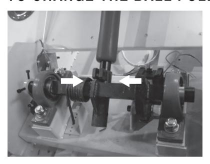
1. Remove the bolt (10mm) from the ball connecting assembly by using 17mm wrench.
