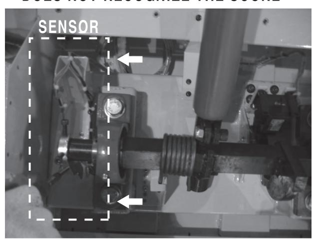
► Change the sensor bracket by removing 2 bolts shown in the picture above.
