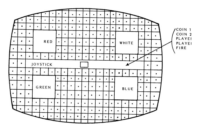
The grid pattern tests your screen for any distortion or convergence.
