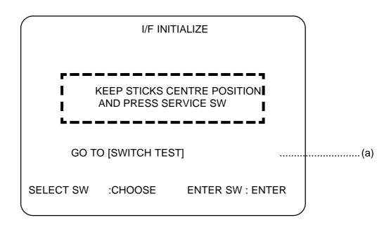
c). Press the Enter button to go to the Switch Test and confirm correct joystick operation. (see next page for test details)
