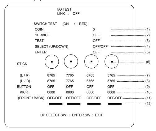
The SWITCH TEST screen displays the status of the switches.
